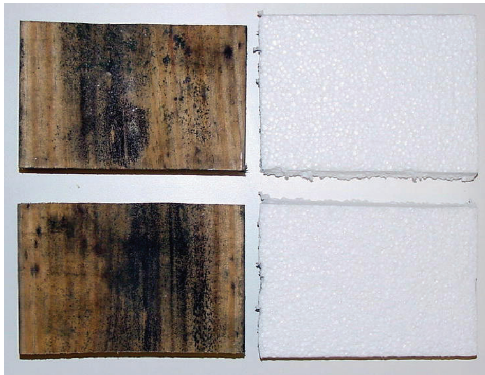
Southern Yellow Pine with Mold Growth
