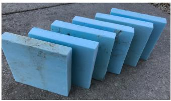
The samples were tested following the industry standard for R-value, ASTM C518, at a mean temperature of 75F.
